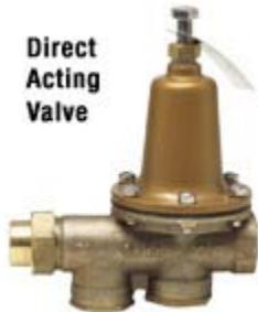
Installed in series and soon after the water meter in homes, commercial buildings, and manufacturing plants, a water pressure reducing valve automatically reduces the pressure from the water supply main to a lower, more sensible pressure.
