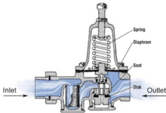
Water entering the valve from municipal mains is constricted within the valve body and directed through the inner chamber controlled by an adjustable spring loaded diaphragm and disc. Even if the supply water pressure fluctuates, the pressure reducing valve ensures a constant flow of water at a functional pressure, as long as the supply pressure does not drop below the valve's pre-set pressure.
