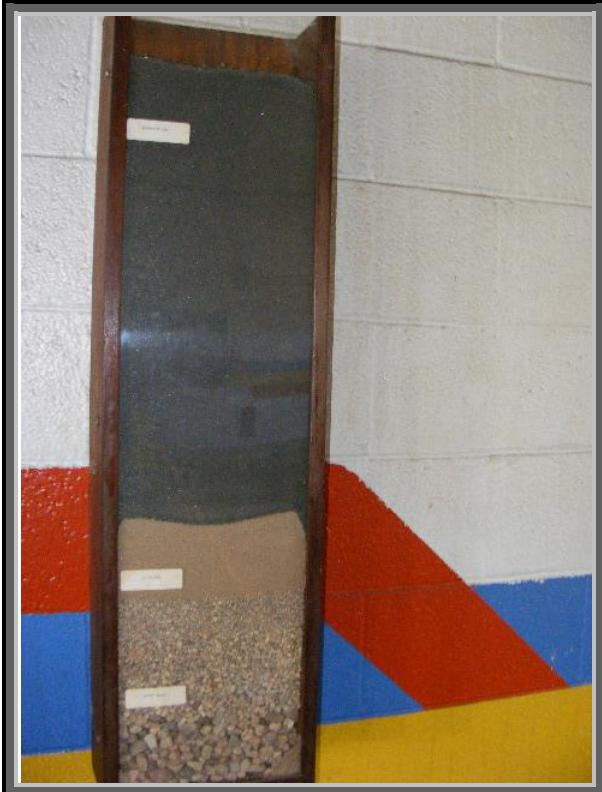
Photograph 19: View of filter material cross section – Anthracite Coal overlying graded sand and gravel.
